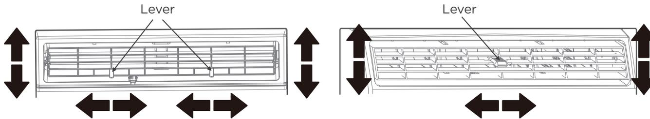
The louvers will allow you to direct the air flow Up or Down (on some models) and Left or Right throughout the room as needed. Pivot horizontal louvers until the desired Up/Down direction is obtained. Move the Lever(s) from side to side until the desired Left/Right direction is obtained.
