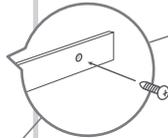
1/8 " (3mm) pilot holes before driving screws. Drive 1/ 2" (12.7mm) locking screws through frame holes into window sash(Only wooden windows:).
