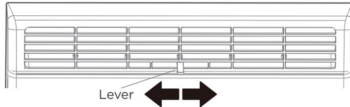
The louver will allow you to direct the air flow Left or Right throughout the room as needed. Move the Lever from side to side until the desired Left/Right direction is obtained.
