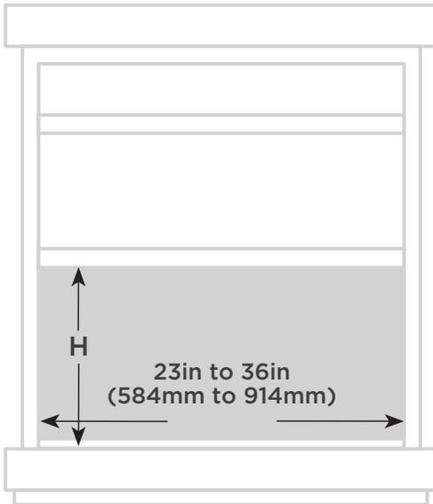
Your air conditioner is designed to install in standard double hung windows with opening widths of 23 to 36 inches (584mm to 914mm).
