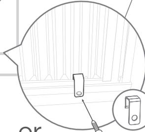
Drive 1/ 2" (12.7 mm) locking screws through the frame lock and into the window sash(Only Vinyl-Clad windows).
