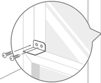
Drive 1/ 2" (12.7 mm) locking screws through the frame lock and into the sill(Only wooden windows).
